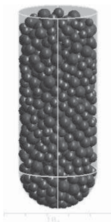
Figure 28.4 A computer simulation of a size 0 capsule filled with pellets with a size distribution of 0.8 and 1.2 mm.
