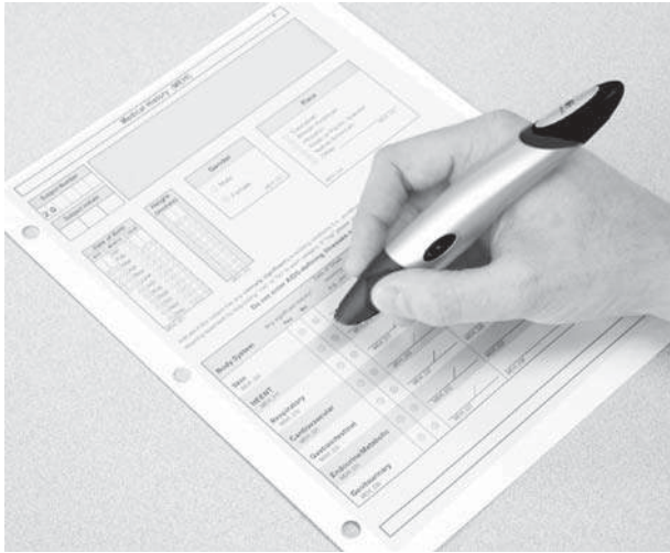
Figure 23.2 The SmartPen™ system is a pen with an optical sensor that records each keystroke on a special form. The pen is docked at a computer or data can be wirelessly transmitted, and data from anywhere in the world are immediately sent for validation. Queries are generated within minutes, closing the feedback loop and markedly reducing query rates as compared to conventional systems.
