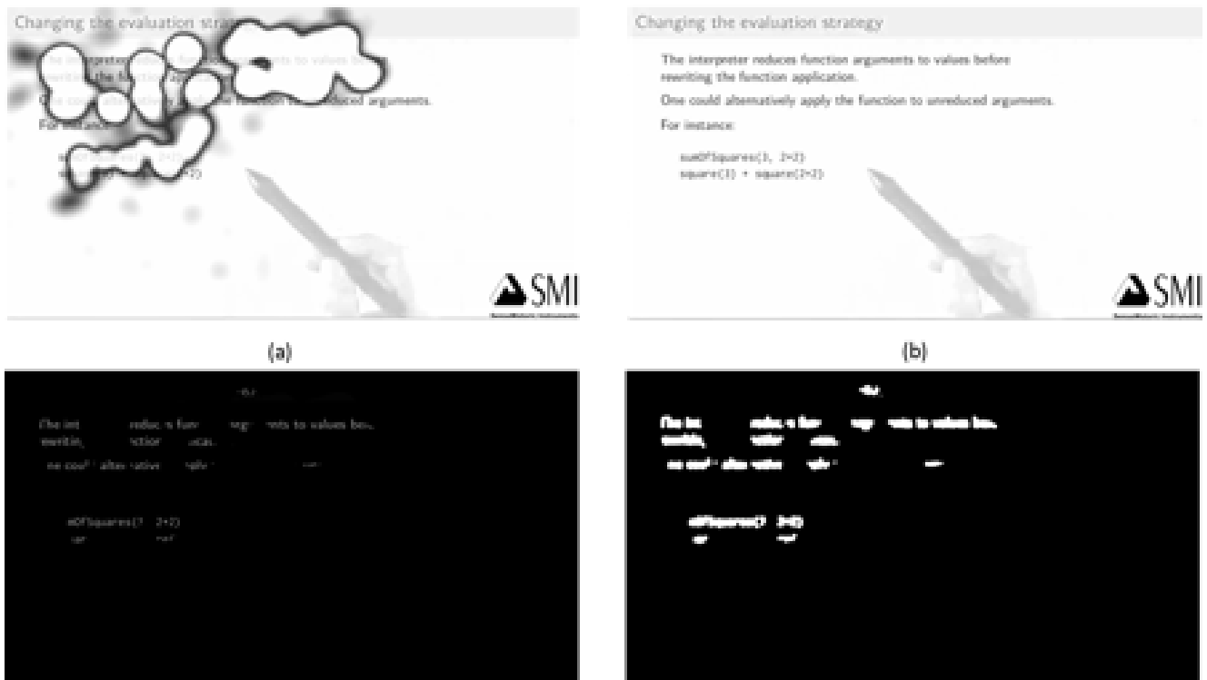
Figure 2: Steps for computing attention points from the heat map. (a) A slide with the 10-second heat-map overlay. (b) A slide (same as (a)) without the heat-map overlay. (c) Resulting on image after subtracting image without the heat-map from heat-map overlaid image. (d) Applying connected component on the image (c) gives us attention points.
