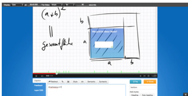
Figure 4. To build a quiz, basic elements are arranged in a layer over the video. These can then be edited in terms of HTML, CSS, LaTeX and the proprietary DSL for checking mathematical expressions.
